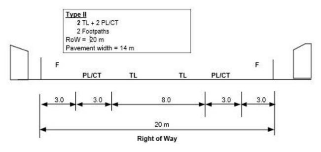
Figure 4: Typical Cross-section for DCRN Roads (with RoW 20m)
