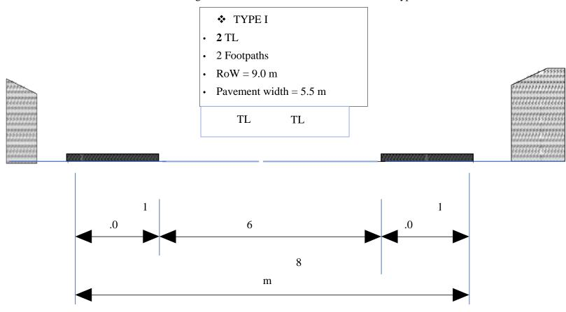
Figure 25: Typical Cross-section for Class C Roads (with RoW 8m)
