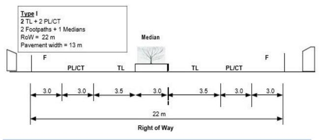
Figure 3: Typical Cross-section for DCRN Roads (with RoW 22m)
