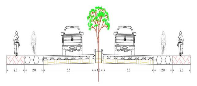
Figure 23: Typical Cross-section for Class A Roads (with RoW more than 20 m)
