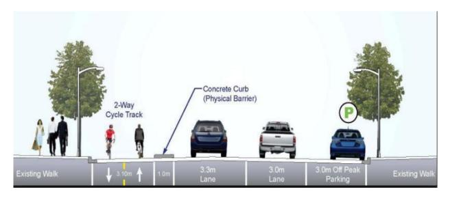
Figure 13: Typical cross section of road with cycle lane
