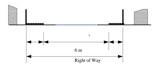
Figure 27: Typical Cross class C Roads (RoW 6 m)
